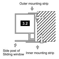
Example of mounting in a wall/section with fixed flange.
