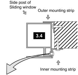
Note that no holes may be drilled in the Sliding window since electrical parts and moving parts are mounted in these sections. The angle strip must therefore be secured to the Sliding window by the manufacturer.
